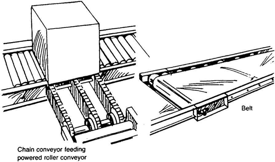
Fig. 38.24 Belt and roller conveyors.
