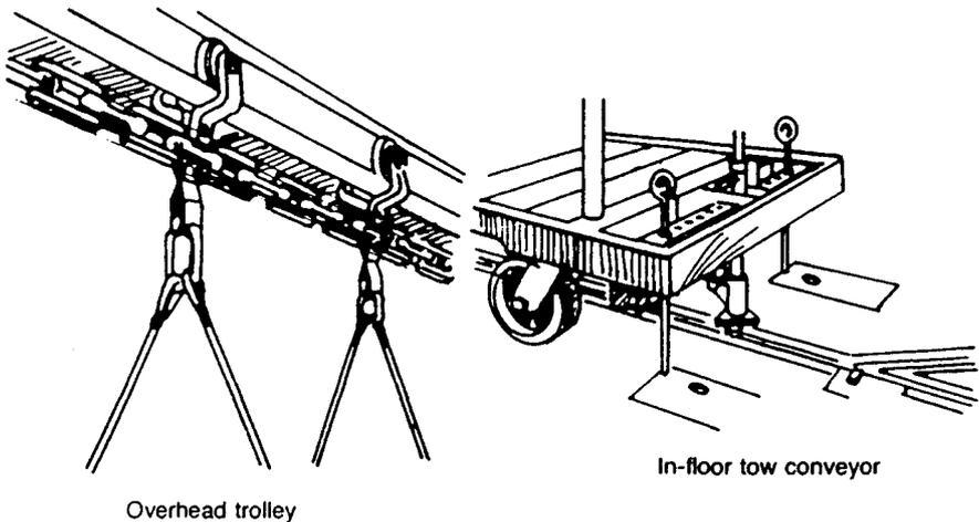
Fig. 38.25 Chain-driven conveyors.
