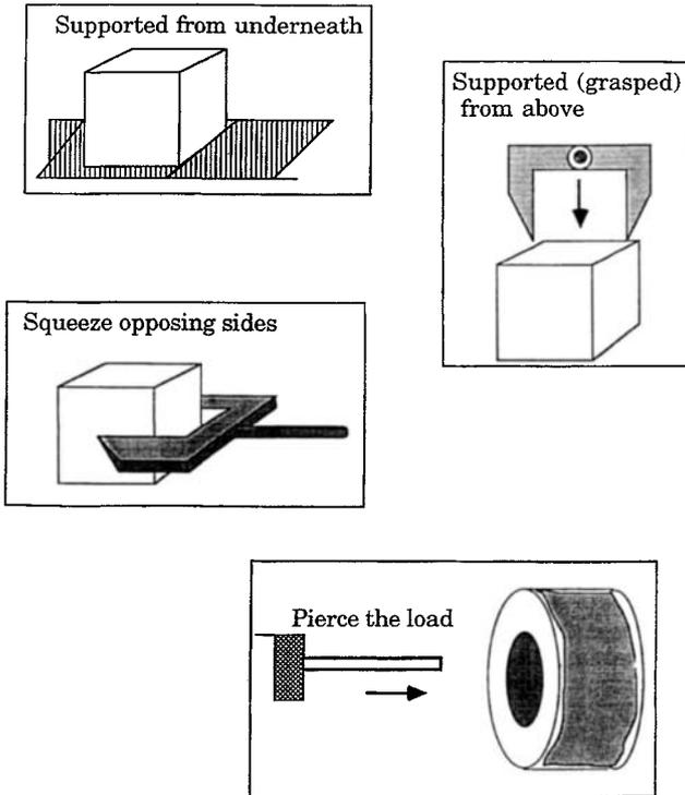
Fig. 38.22 Ways to handle a load.
