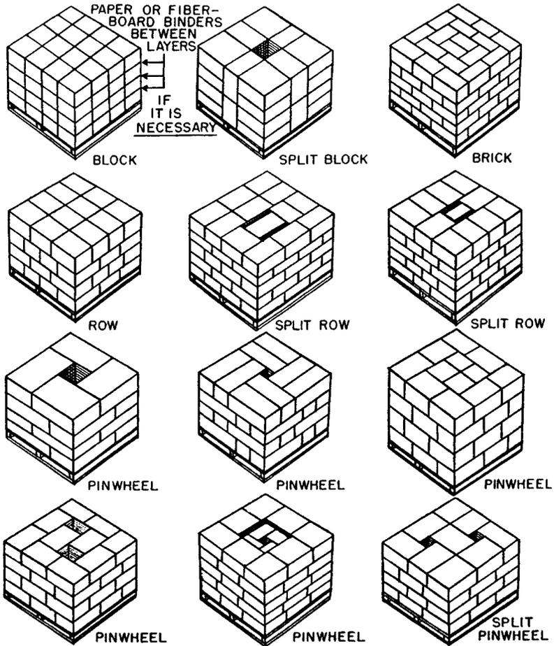
Fig. 38.20 Example pallet-loading patterns.
