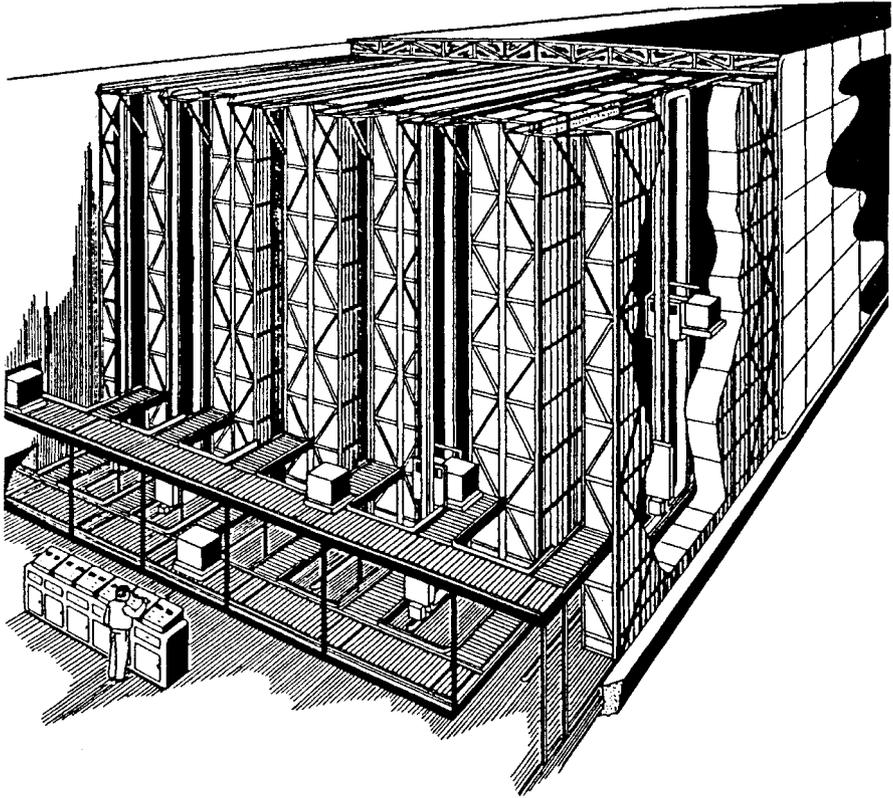
Fig. 38.32 Automated storage and retrieval system.
