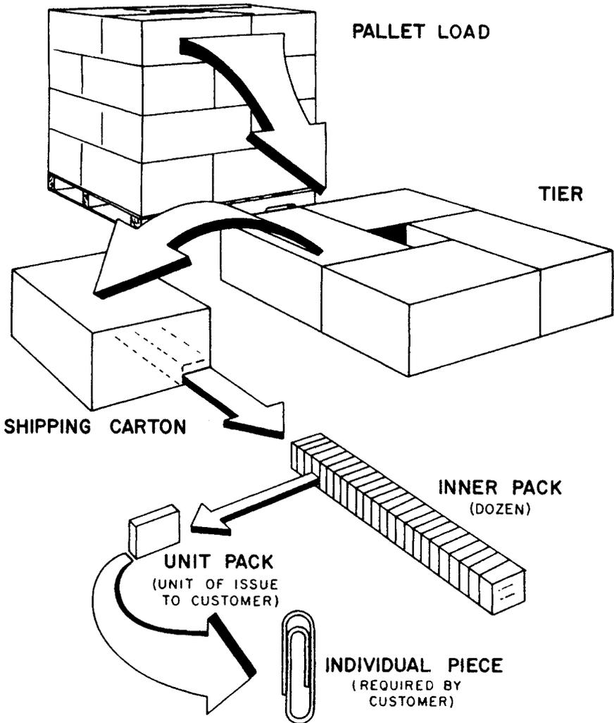
Fig. 38.19 Unit load design.
