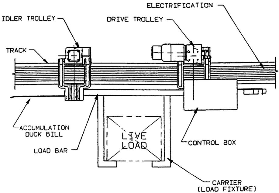
Fig. 38.27 Automated electrified monorail.
