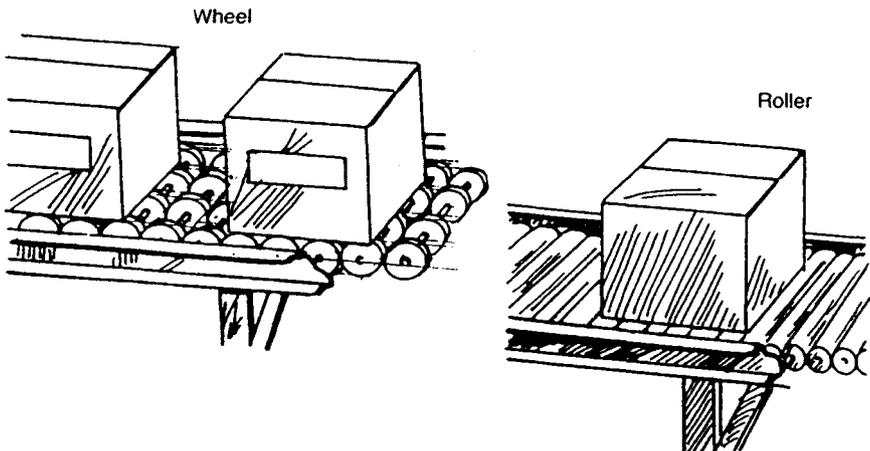
Fig. 38.23 Gravity conveyors.
